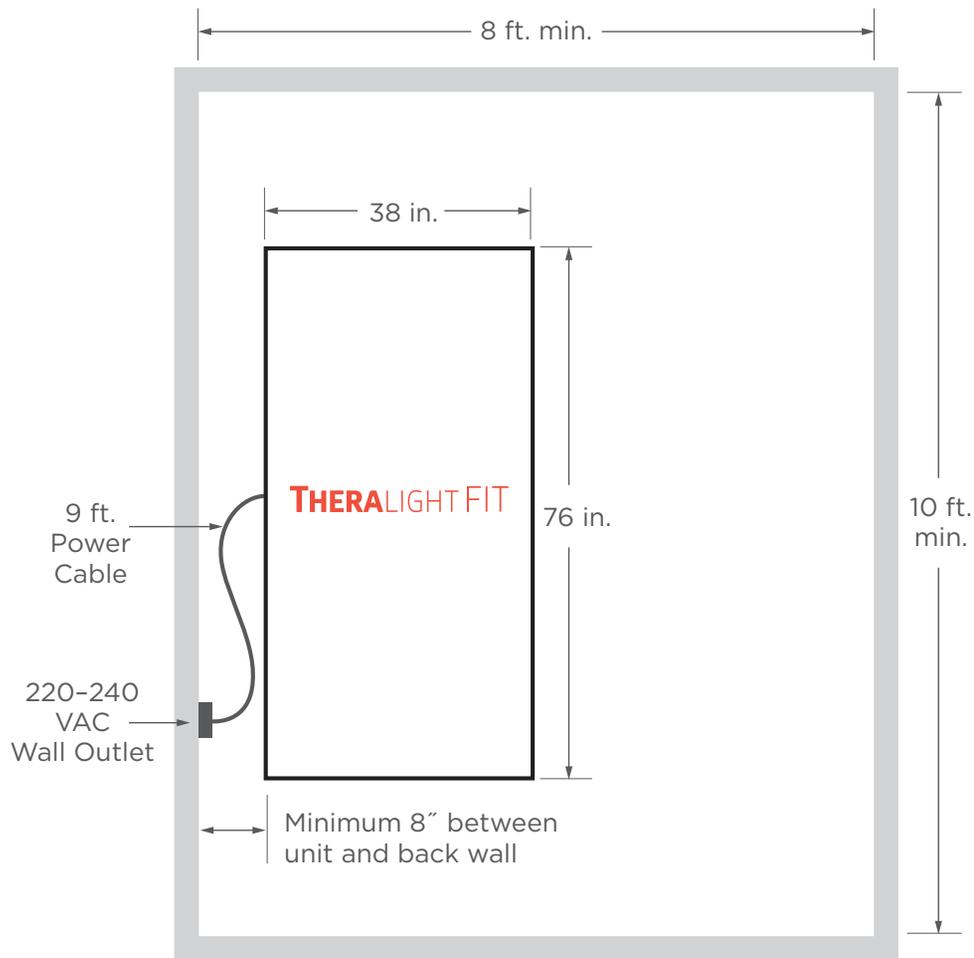
**PLEASE NOTE:** Failure to adhere to these minimum space requirements can result in compromised performance and/or damage to the TLFIT, thereby voiding its warranty.
