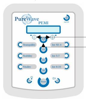
Increasing the digit positioned below the cursor by pressing the right arrow-key, or to lessen it via the left arrow-key.
