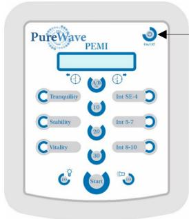
To switch on the device please press the On/Off key.
