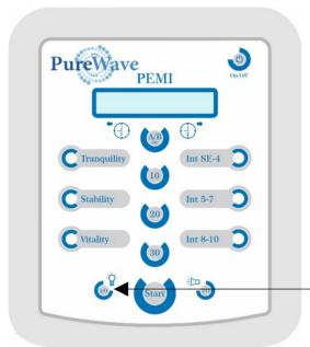
The backlight status may be checked by simply pressing the I/O-key
