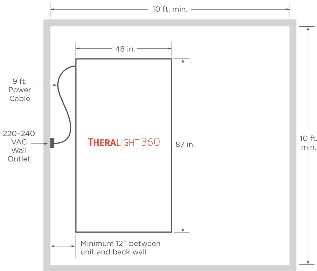
**PLEASE NOTE:** Failure to adhere to these minimum space requirements can result in compromised performance and/or damage to the TL360, thereby voiding its warranty.
